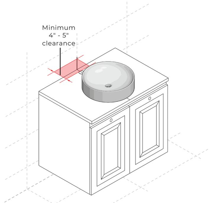
**IMPORTANT:** For wall-mounted faucets, disregard the 4-5 inch minimum space requirement. Instead, adjust the sink location to fit the faucet's reach, ensuring the spout extends to a position that prevents splashing. Follow the manufacturer's installation guide for precise steps.
